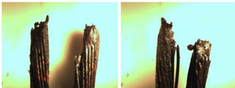
Figure A90: Direct Flame, Multi-strand 18-2, Non Energized (Test No. 37)
