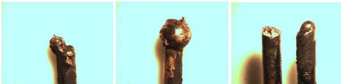
Figure A66: Direct Flame, ROMEX 14-2, Energized (Test No. 66)
