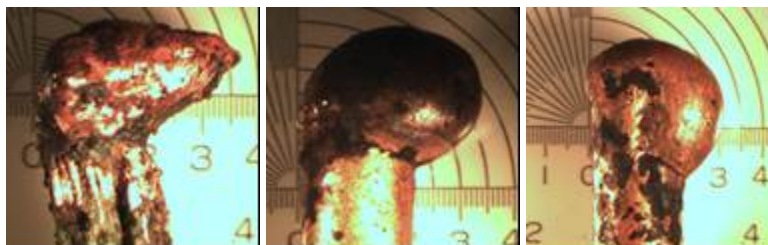
Figure 23: Beads Produced with Radiant Tunnel Exposure (16-gauge: NE, 12-gauge: E (center) and L)
