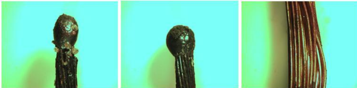
Figure A77: Direct Flame, Multi-strand 16-2, Non Energized (Test No. 23)
