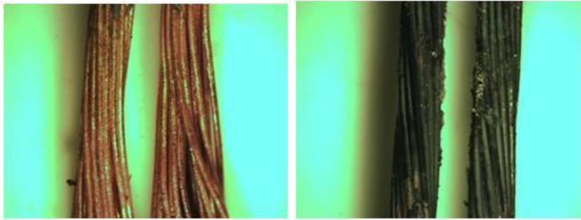
Figure A73: Direct Flame, Multi-strand 16-2, Non Energized (Test No. 19)
