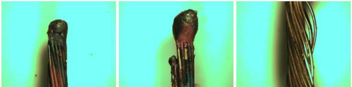
Figure A74: Direct Flame, Multi-strand 16-2, Non Energized (Test No. 20)
