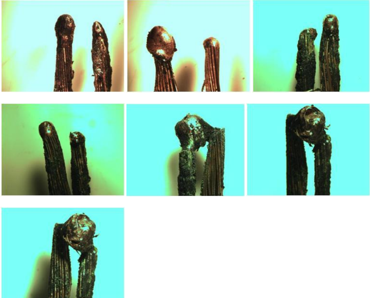
Figure A104: Direct Flame, Multi-strand 18-2, Loaded (Test No. 54)
