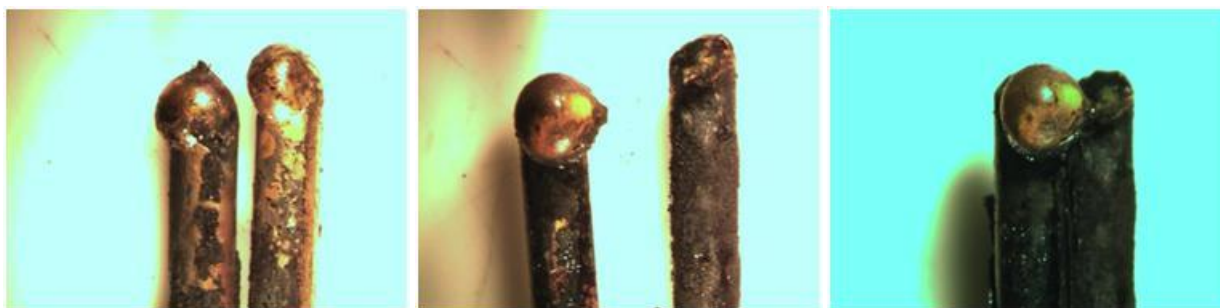
Figure A71: Direct Flame, ROMEX 14-2, Loaded (Test No. 71)
