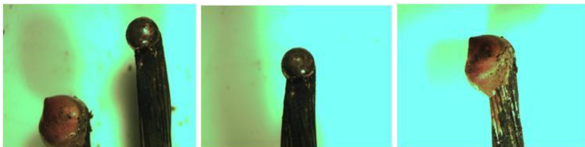
Figure A80: Direct Flame, Multi-strand 16-2, Energized (Test No. 26)
