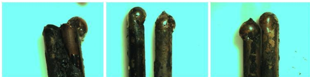
Figure A72: Direct Flame, ROMEX 14-2, Loaded (Test No. 72)
