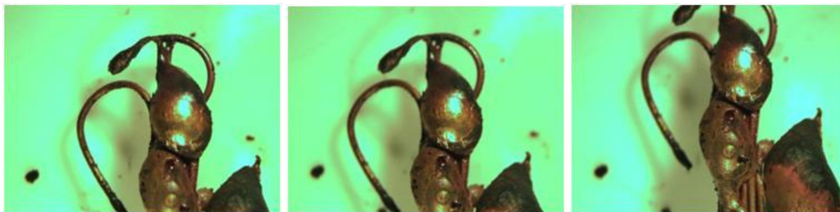
Figure A80: Direct Flame, Multi-strand 16-2, Energized (Test No. 26)
