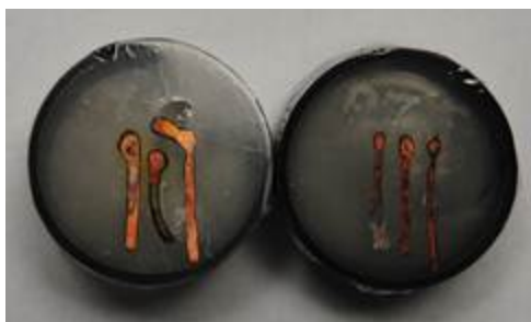
Figure 26: Mounted Samples (Cut and Etched)
