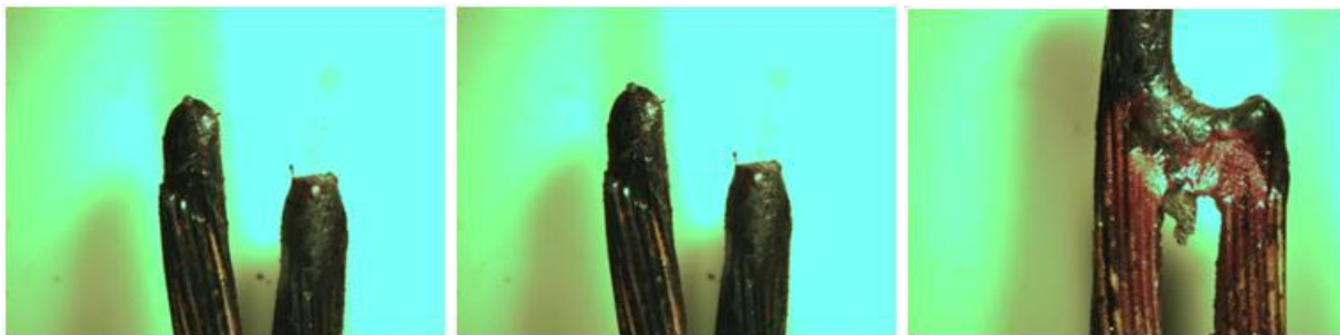
Figure A77: Direct Flame, Multi-strand 16-2, Non Energized (Test No. 23)
