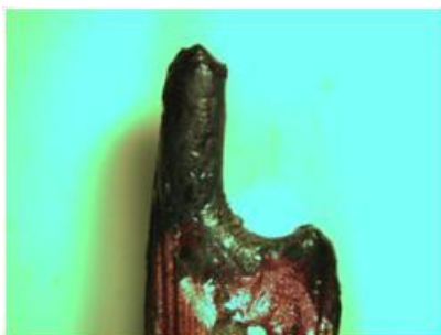
Figure A78: Direct Flame, Multi-strand 16-2, Non Energized (Test No. 24)
