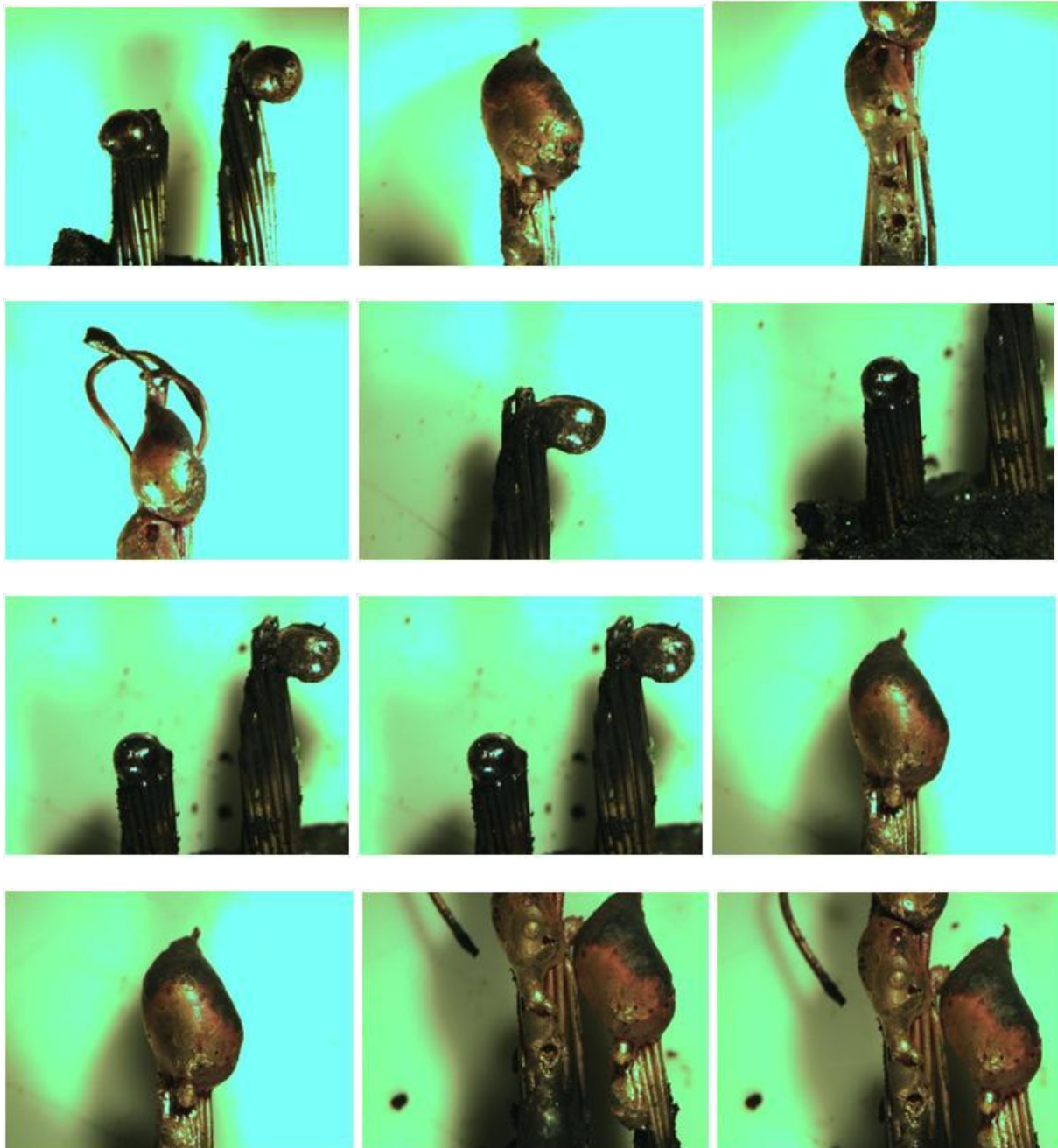
Figure A79: Direct Flame, Multi-strand 16-2, Energized (Test No. 25)
