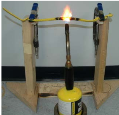
Figure 2: Direct Flame Testing Setup
