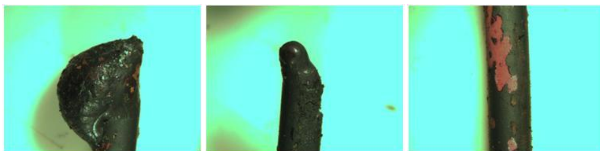
Figure A44: Direct Flame, ROMEX 12-2, Non Energized (Test No. 5)
