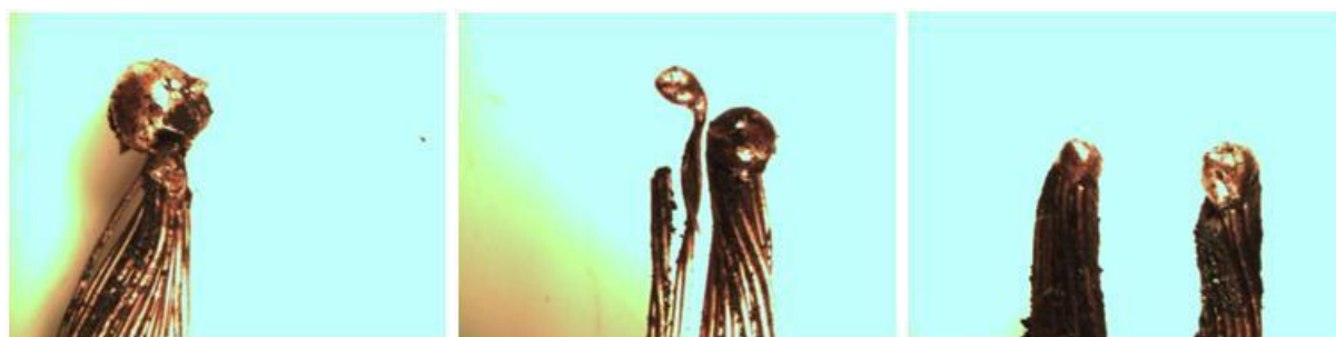
Figure A97: Direct Flame, Multi-strand 18-2, Energized (Test No. 46)
