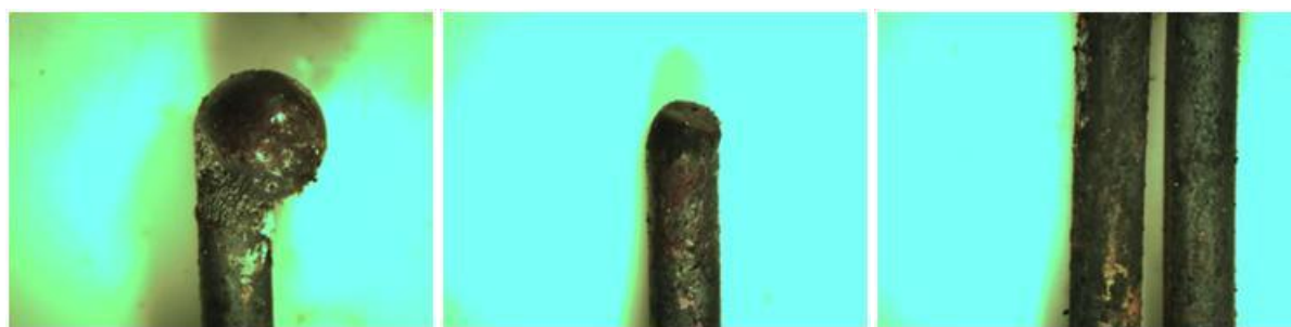
Figure A59: Direct Flame, ROMEX 14-2, Non Energized (Test No. 57)
