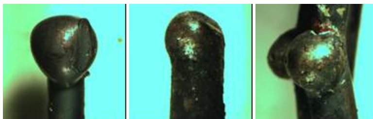
Figure 22: Beads Produced with Direct Flame Exposure (12-gauge: NE, E (center), and L)
