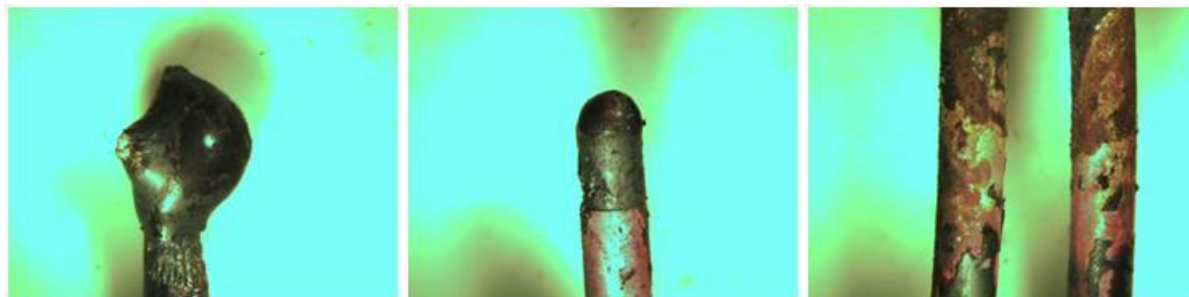
Figure A58: Direct Flame, ROMEX 14-2, Non Energized (Test No. 56)
